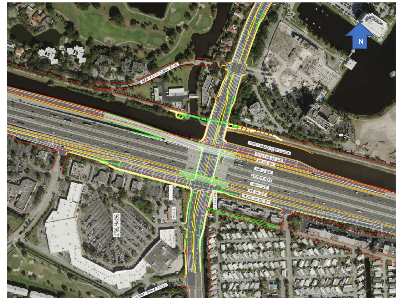
Figure 3-28: Modified Diamond Interchange with Overpasses Concept
