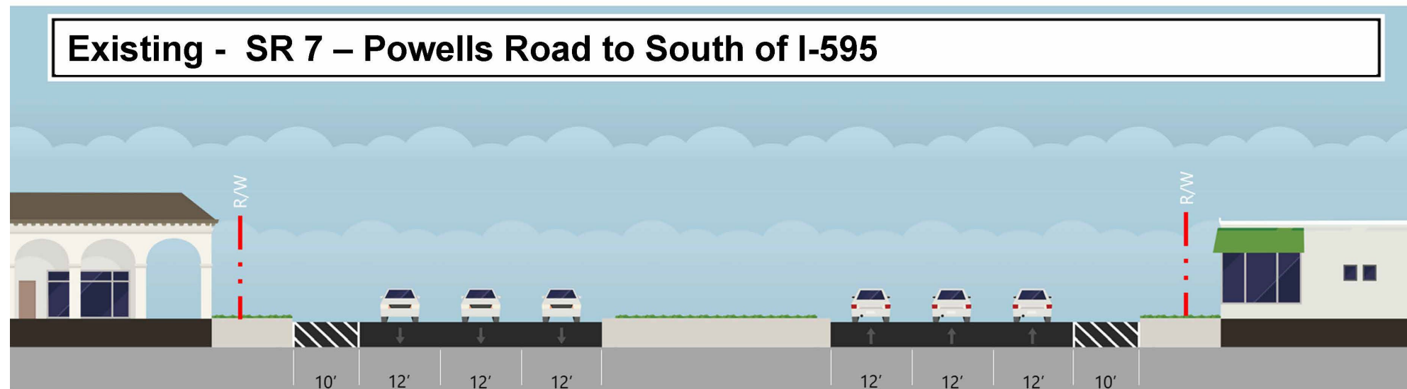
Figure 3-44: SR 7 Existing Typical Section, Powells Road to South of I-595
