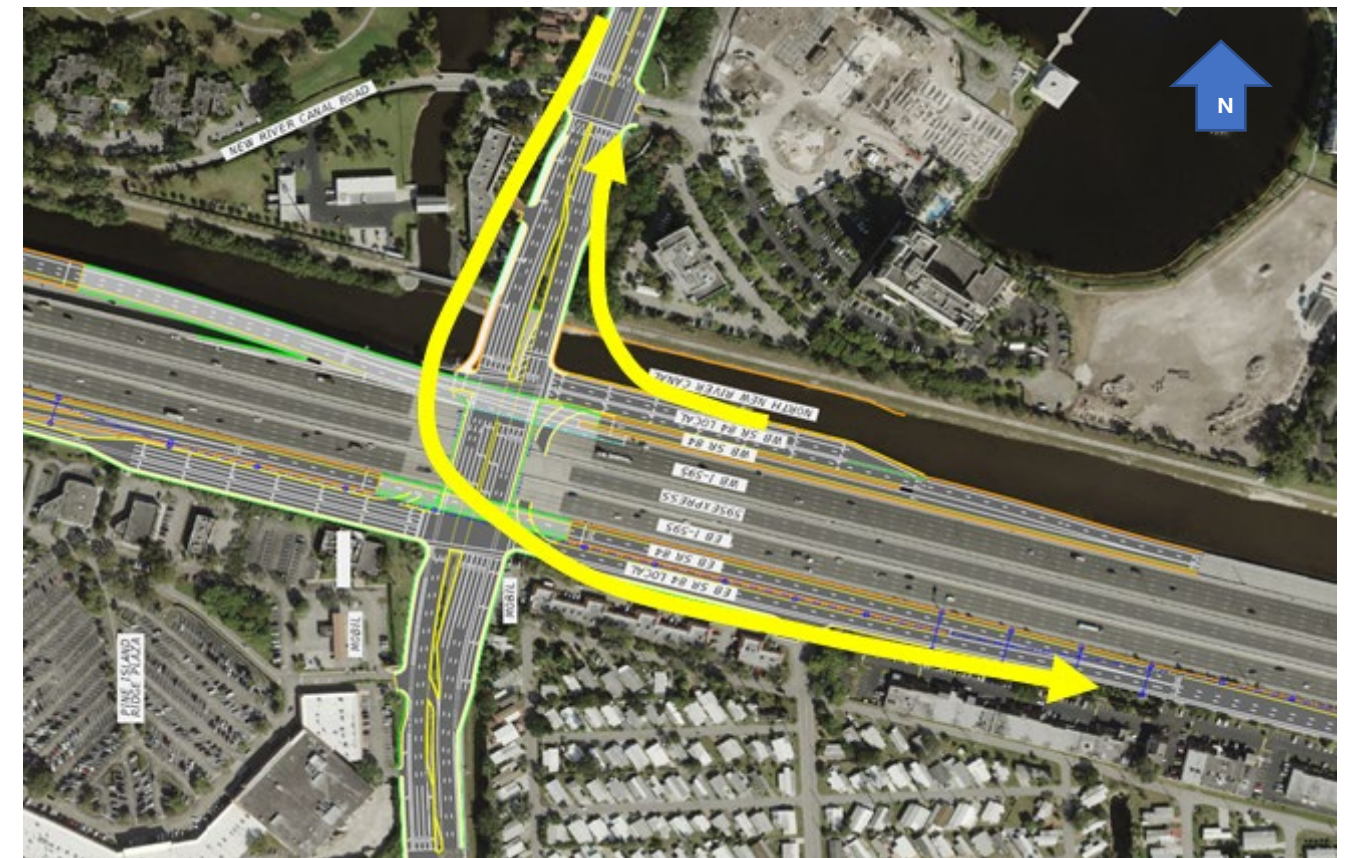
Figure 3-27: Modified Diamond Interchange with Overpasses and Flyover Concept
